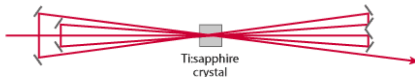
Figure 3: Signal path in a multipass amplifier. The pump beam is not shown.
