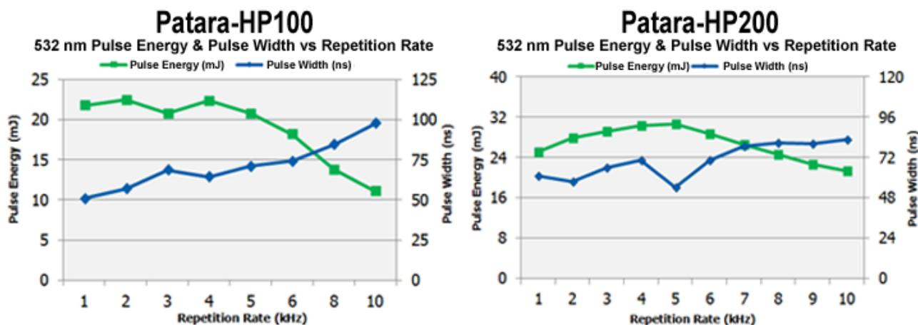
Figure 4: 532nm pulse energy and pulse width WRT repetition rate for Patara-HP100 and Patara-HP200 laser systems. Patara-HP200 was optimized at 5 kHz for 5 kHz-10 kHz repetition rate operation.
